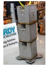
Overload testing was performed on the HIBSX 24 x 24-inch with a capacity of 1300 lbs using three 1,000 lbs test weights. The scale was operational and tested accurate with test weights even after this grueling test.
